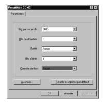
Configure communication parameters, 9600 bauds, no parity, 8 data bits, 1 stop bit, no flow control and validate. The PC is in terminal mode, connect to device by plugging in the RS232 link cable. Measure is now displayed and to access at the configuration, press on "C" key.
